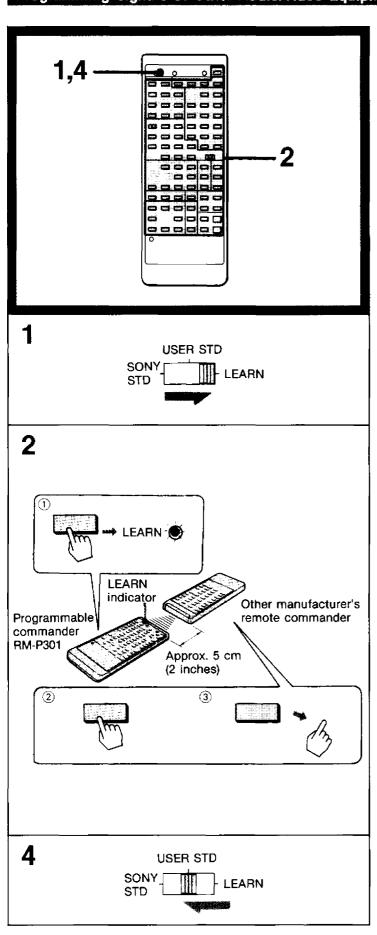
The RM-P301 learns various functions of other remote commanders emitting infrared rays and allows you to control most of audio and video equipment from a distance.
